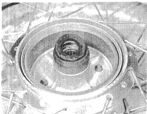
11.2a Oil seal is in front of wheel bearings, will be displaced before ...
