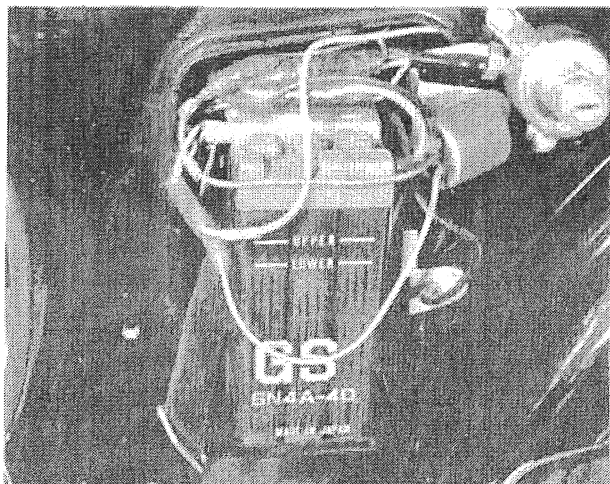
5.4 Disconnect battery and remove from machine
