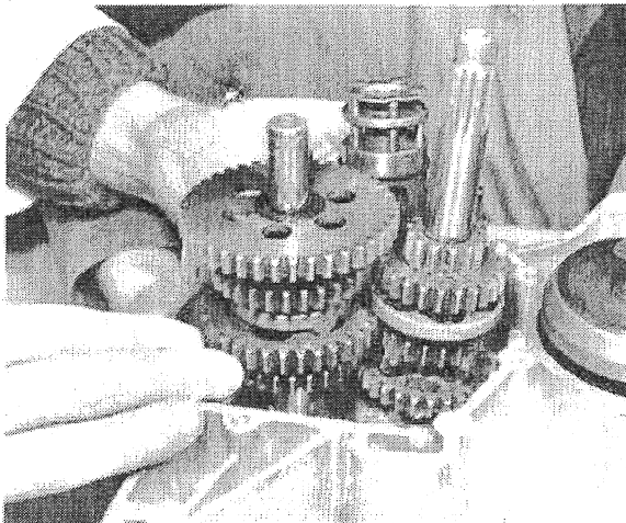
31.2a Mesh gear trains prior to assembly and fit with gear selector drum
